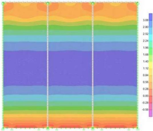
Figure 10: Maximum Tensile Glass Stress – Windward Load
