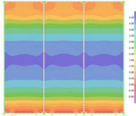
Figure 11: Maximum Tensile Glass Stress – Leeward Load
